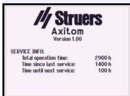
Axitom contains software offering valuable information to the user about the status of the machine.
