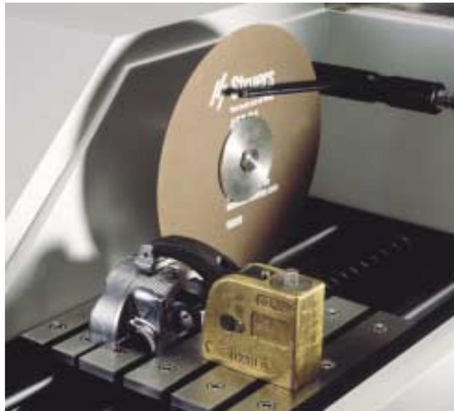
Struers vertical clamping device on the movable cutting table of Secotom-10
