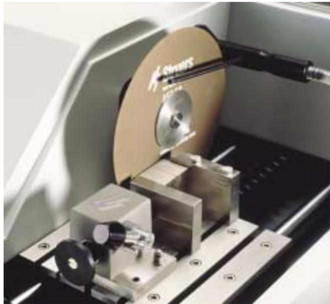
*Struers quick-clamping device on the movable cutting table*
