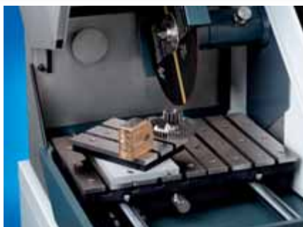
The cutting table is provided with 10 mm T-slots allowing various clamping tools to be used.
