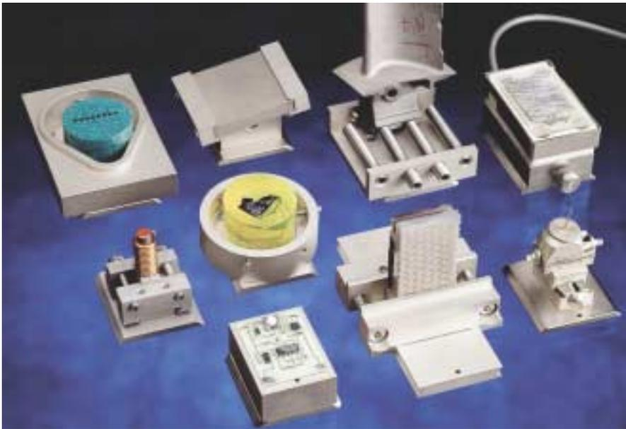
*A wide range of specimen holders can be used on Secotom-10*
