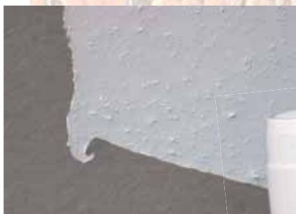
Edge of aluminium specimen, mounted in LevoFast, DIC, 200x
