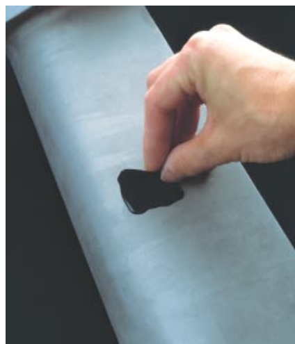
An operator peels off the cured replica
