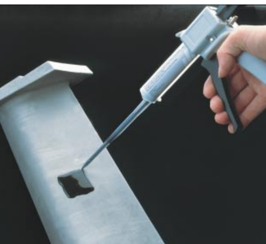
An operator dispenses RepliSet onto a sample
