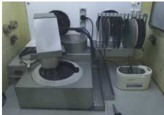
The RotoPol polisher/grinder inside the hot cell
