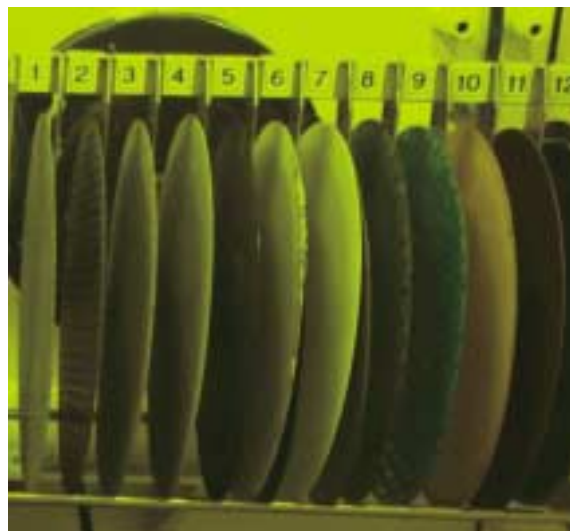
The use of the magnetic grinding discs from the MD-System simplifies the preparation process. (Photographed through observation window)
