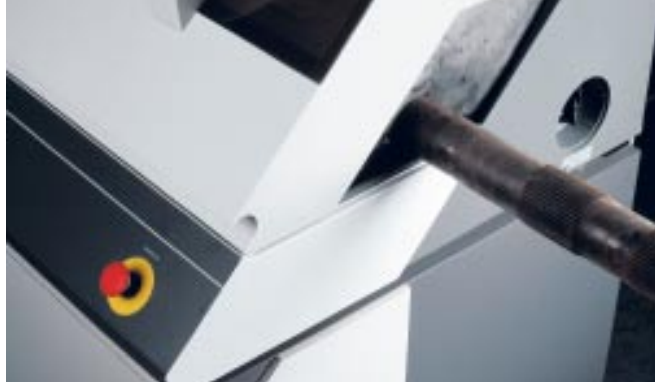
Cutting of very long, protruding workpieces using optional rubber curtains
