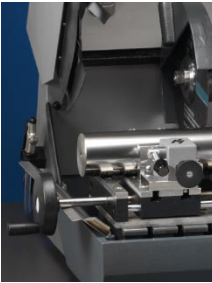
The adjustable cutting table enables parallel sectioning
