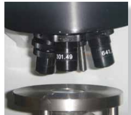
The automatic turret holding four positions facilitates lens and indenter exchange and ensures correct lens selection
